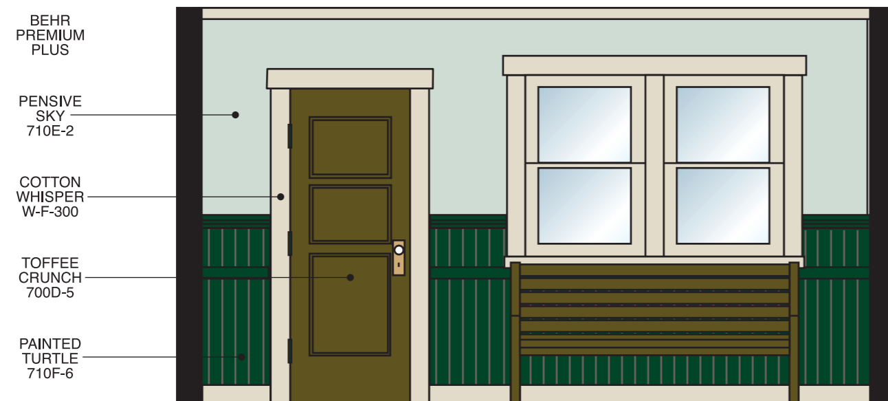
EAST INSIDE ELEVATION OF ENTRY HALL
